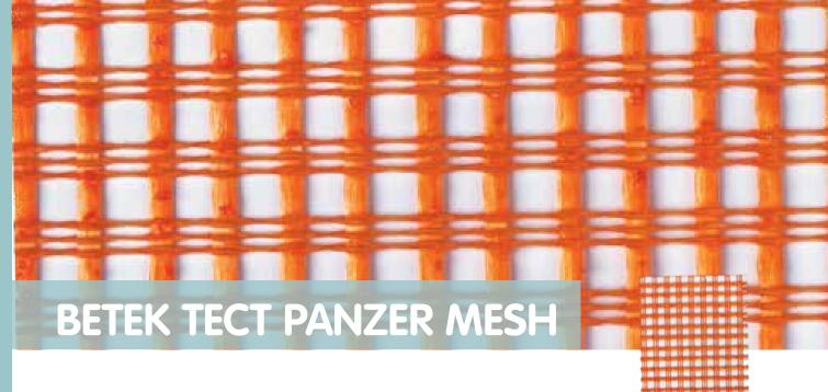
Betektect Panzer Mesh is a special coated glass-fiber mesh with 340 g/m² weight, 5.0 x5.5 mesh size and alkali resistance. Used as a bearing element in surfaces requiring higher strength like entrance floors, parking areas and waste storage areas.
